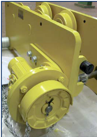
29/06 APH. with hand geared trolley
