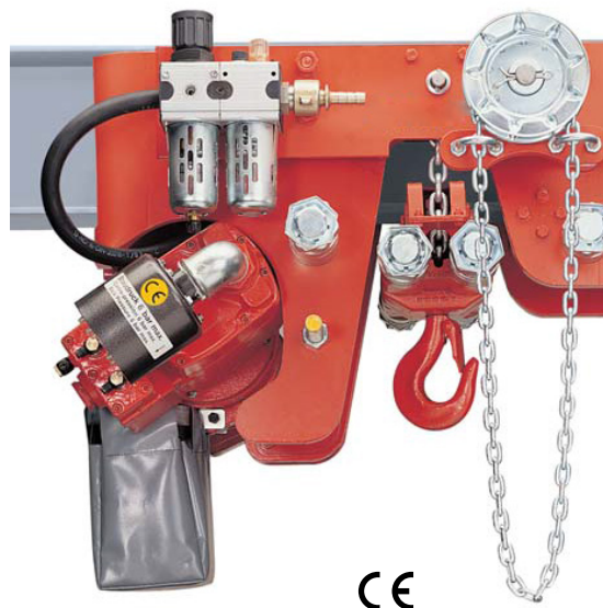
Zinc plated high quality RUD load chain with improved tolerances to achieve smooth running and to reduce wear
