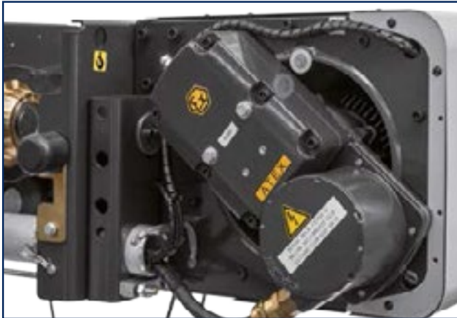
Hoist gear and hoist limit switch designed according to ATEX
