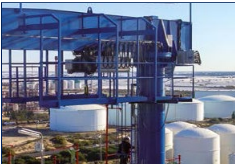
Pillar jib crane 3.2 t with electric wire rope hoist NOVAex
