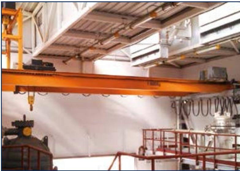
Double girder overhead travelling bridge crane 10 t with electric wire rope hoist NOVAex
